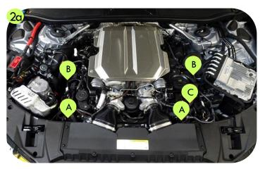
Harness Section A – Turbo Boost Pressure Sensor (Right-Left) – Route section A down towards the front of the engine on both the left and right hand of the engine. Disconnect the turbo boost pressure sensor connecter and wire in series both the PCM wiring harness section labelled A. See figure 3a & 3b for assistance.
