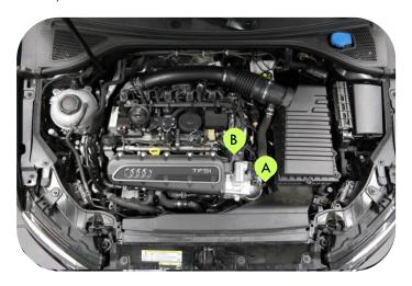
**Step 3 – Wiring Harness Installation:** Lay wiring harness over engine bay and route the labelled harness sections to there respective connection points, using Step 2's images for reference.
